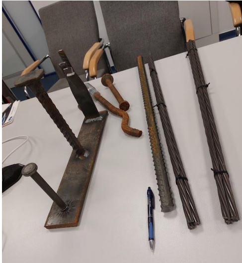
Types of reinforcement
